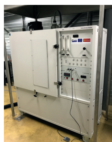
Analysis of smoke emitted during combustion
